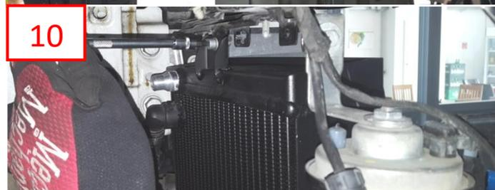
*Insert the front mounted WT radiator on the original mounting points (11) and connect its hose connections. Fix the mounting screw of the lower subframe made of plastic (6).*
